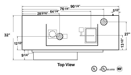
The oven's minimum clearances from combustible materials are 2" on left side, 18" on right, 18" on top, 36" from front, and 2" on back. Floor may be constructed of a combustible material. (Note: minimum clearance dimensions are from the oven cabinet, not from component cover.)
